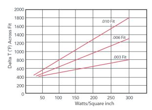
Figure 6: Temperature di erential across fit as a function of watt density. Source: Backer Hotwatt
