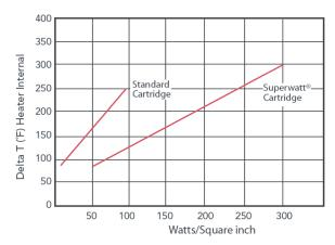
Figure 7: Internal temperature differential for standard and Superwatt=cartridge heaters as a function of watt density. Source: Backer Hotwatt
